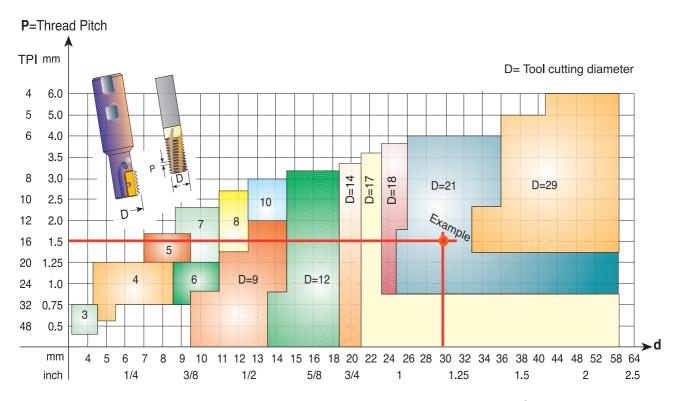
Any tool with a small cutting diameter can produce large diameter threads.
